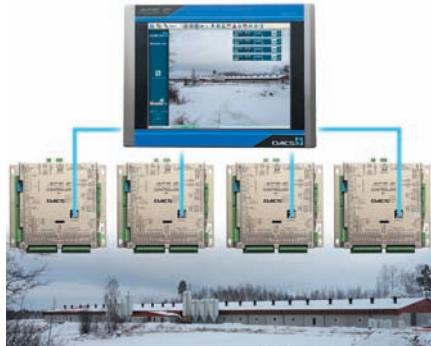
A building with four houses with main supply board where the ACSnet touch server is placed. From this touch screen all four ACS6 computers are operated.
