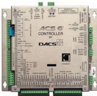
The core of the control system is the ACS6 controller. The powerful ARM CPU running Linux OS and interface with a wide range of inputs and outputs makes this controller able to handle the most advanced types of modern poultry production.
