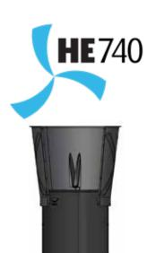
The HE740 with butterfly damper on top of the chimney is a high efficiency and energy saving exhaust unit for livestock facilities. With a specific power consumption of 25.5 W/1000 m3/h, the exhaust unit is "best practice" in the industry and takes a significant lead over competing products.
