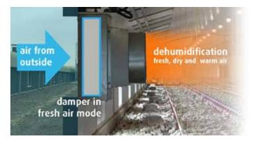
When dampers are open the unit serves as a heat exchanger and provides superior humidity control and ample supplies of preheated fresh air. The air entering the building is warm and will not cause draft or condensation. The air leaving the unit is extremely dry and will absorb moisture quickly and efficiently.
