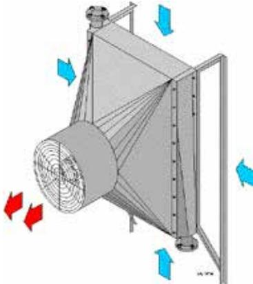
The DACS all steel, galvanized-radiator produces plenty of dry, hot air without any risk of sparks flowing. The heating surface and the assembly rack on the radiator are fully hot dipped galvanized and thus protected against the aggressive environment in a poultry house.
